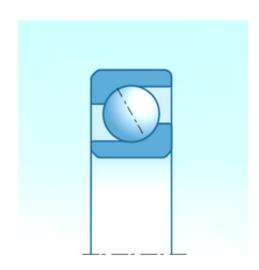
25,000 mm x 52,000 mm x 15,000 mm 25,000 mm x 52,000 mm x 15,000 mm SNR 7205BGA angular contact ball bearings
